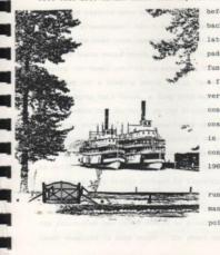
before she sank, and she was back in service a few weeks later (Downs 1967, 7). The paddlewheel had a very practical function in that it needed Just a few Inches of water to produce very powerful thrust. The construction and maintenance costs of such vessels was low in comparison with vessels of conventional design (Estabrooks 1968, 28).
